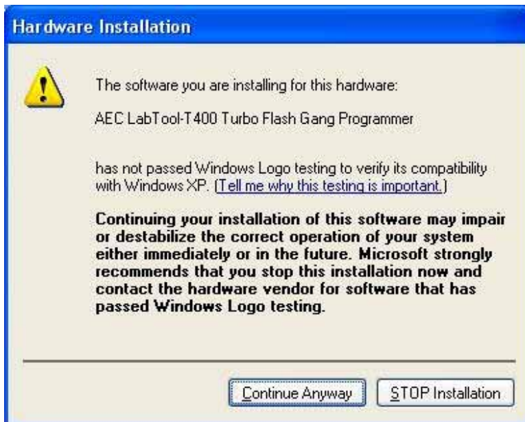
Fig2-4 : Press “Continue Anyway”. If you select the other button, the O.S. will has a wrong “!USB Device” in your PC.
