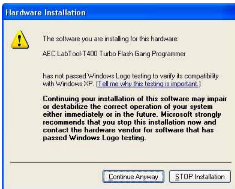
Fig6-4 : Press “ Continue Anyway” . If you select the other button, the O.S. will has a wrong “!USB Device” in your PC.
